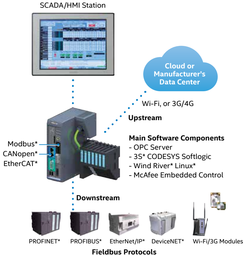
Figure 2. Simplified Architecture Connecting Field Devices to SCADA/HMI, the Cloud or Data Center
