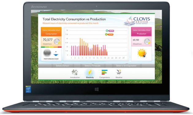
Figure 2. Dashboard created through the use of Lucid BuildingOS* trend analysis application
